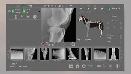
Just a single screen for acquisition process including FPD, X-ray and APR control tools
